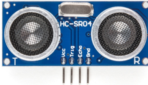
Figure 5: HC-SR04 Ultrasonic Sensor Module
